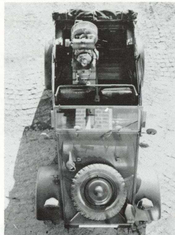
Above: The Type 82 with the 822 Body as a two-seat siren car. The engine-driven siren was installed in place of the rear seat.
