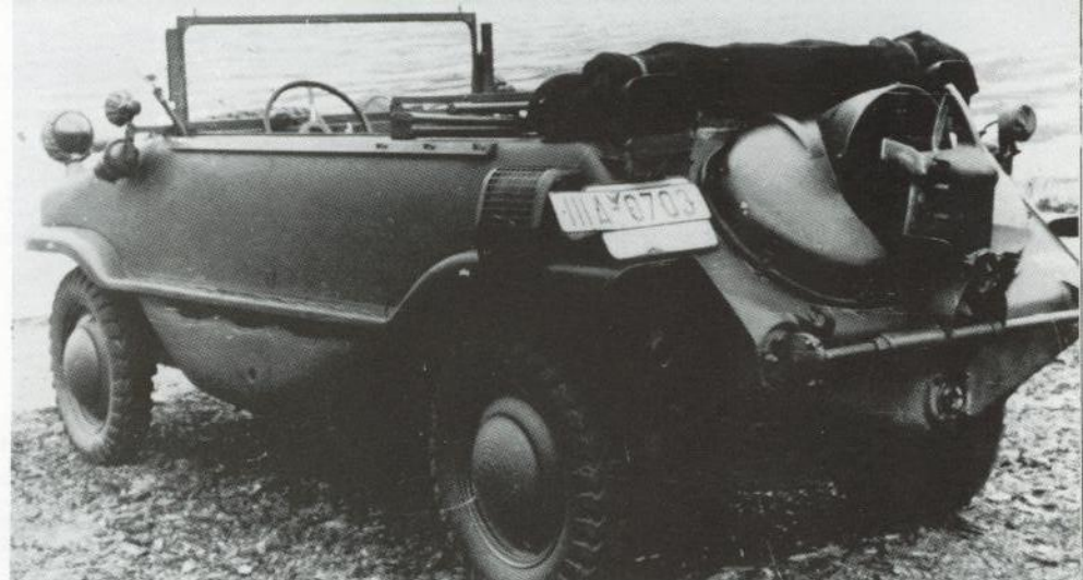
Above: A pre-production model of the Type 128 Schwimmwagen, recognizable by its different engine cover, which also enclosed the propeller, and the special intake and exhaust installations. Here, in contrast to later models, the shaft around which the propeller was lowered extends across the entire width of the vehicle. Below it is the clutch coupling of the intermediate shaft to the motor, which engaged the propeller shaft.
