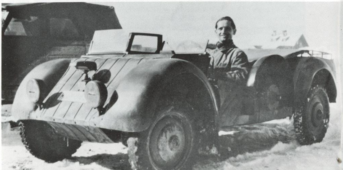
A later prototype of the Geländewagen (Cross-country Car) 62, also called the "Stuka." In contrast to the vehicle illustrated on the facing page, it already displays the angular superstructure with the typical structuring of the sheet metal. The mount for the spare tire (here removed) was located on the side of the vehicle. Note that the windshield is lower on the driver's side than on the passenger's side.
