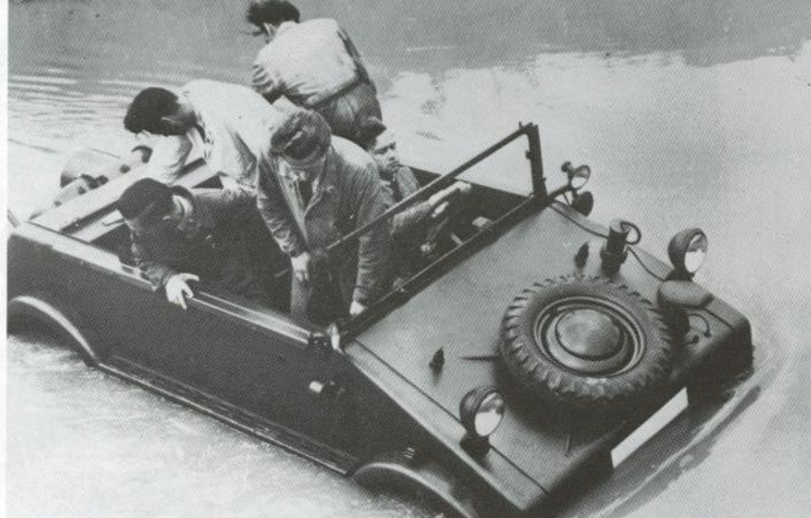
Above: Porsche conducted trials to determine the amphibious abilities of the Kübelwagen early in the development program. Here one such sealed vehicle is seen undergoing a test in the Stuttgart firm's fire pond.
