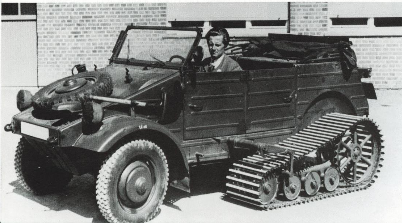
These three photographs show the different running gear arrangements tested for snow tracks. The drive sprocket was always installed on the rear axle. The track drive extended forward to about mid-vehicle, where it was usually attached to a supplementary swivel arm.
